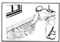
3/8" brads can also be used to blind nail and no pre-drilling is needed. Continue the installation using an engineered wood-flooring stapler, using recommended staples. Staple flooring 1" to 2" from ends and every 4" to 6" along the edge tongues. See notes in floating section for end joint spacing and starting additional rows.
