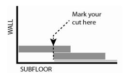
Next, place the marked plank on a cutting board. Using a carpenter square as a guide, score the pencil line carefully with a sharp knife, then break/snap (or cut) the plank or tile along the score mark.
