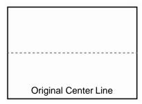
To avoid small narrow planks along the walls, divide the distance from the center line to the wall by the plank or tile width. If the remainder is less than 3 inches, adjust the center line one half width of a plank in either direction. This will provide a balanced layout with larger cut pieces at the wall.
