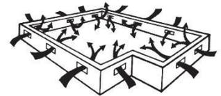
**Note:** To increase reliability, sub-floor appropriate moisture testing should be performed after the HVAC system has been in operation for a **minimum of 14 days**. Excess moisture on any flooring substrate if not identified and corrected prior to installation will cause floor covering failure. **Our Warranties DO NOT cover** any problems due to moisture levels that exceed these guidelines
